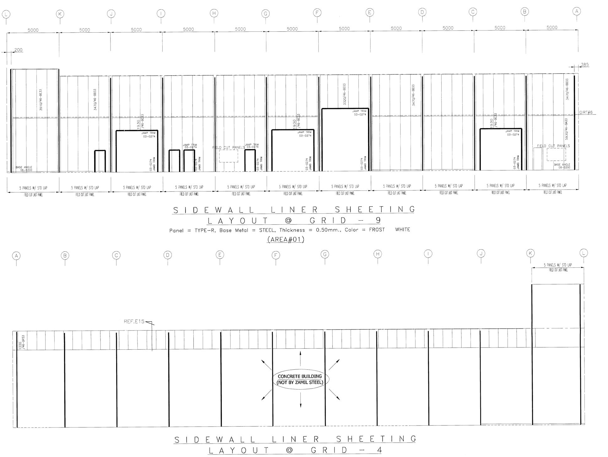
Panel = TYPE-R, Base Metal = STEEL, Thickness = 0.50mm., Color = FROST WHITE (AREA#01)
